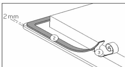
Glue the seal (2) two millimetres from the outer edge of the glass after removing the protective film (3).
